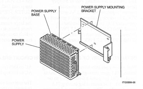
Note: Removal of this device varies with machine configuration and the location of the power supply within the machine.
